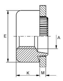
Female thread A = M12Height K = 10.0Outer diameter E = 25.0Plate thickness = 3.5 to 3.7
